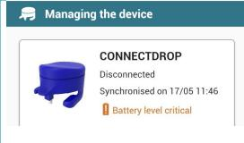
→ Your CONNECTDROP® device has a battery life of less than one month.
